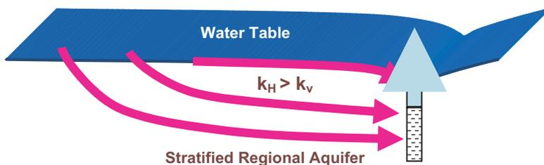
Anisotropy ratio is low enough so that currently (circa 2002) the existing pumping at depth forms a cone of pressure depression at the water table
